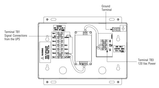
Figure 5-7. Remote Monitor Panel II and Relay Interface Module II Terminal Locations
